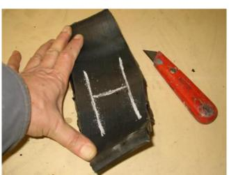
This is the cunning part. Spread open the tyre section and mark an "H", as shown in fig 5. Make the three cuts of the "H" right through the tread, taking care not to sever your thumb at the same time! That completes the "silencer".
