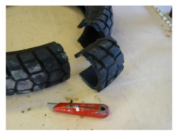
Fig 4 shows one section removed; carry on cutting off more sections if you're making a set.
