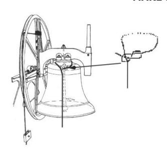
Position yourself comfortably on one side of the bell. Pass one end of the rope around the top of the bell under the headstock making a loop.
