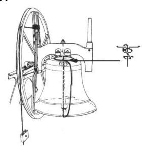
Bring the loose end of the rope to your side of the bell and pass the end through the loop that you made at the beginning. Pull the rope towards you very tightly. Secure it with two half hitches as shown.
