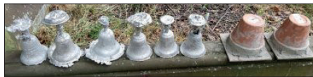
The six cast bells. The two still to be cast show the 'cope' made from flowerpots
